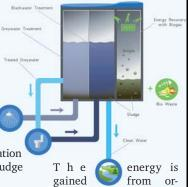
ganic material, the wastewater treatment sludge as well as biowaste and residuals. Using the biogas out of this sludge and waste, not only the energy bill is reduced to a minimum, but also the CO balance of the whole system is significantly improved.
